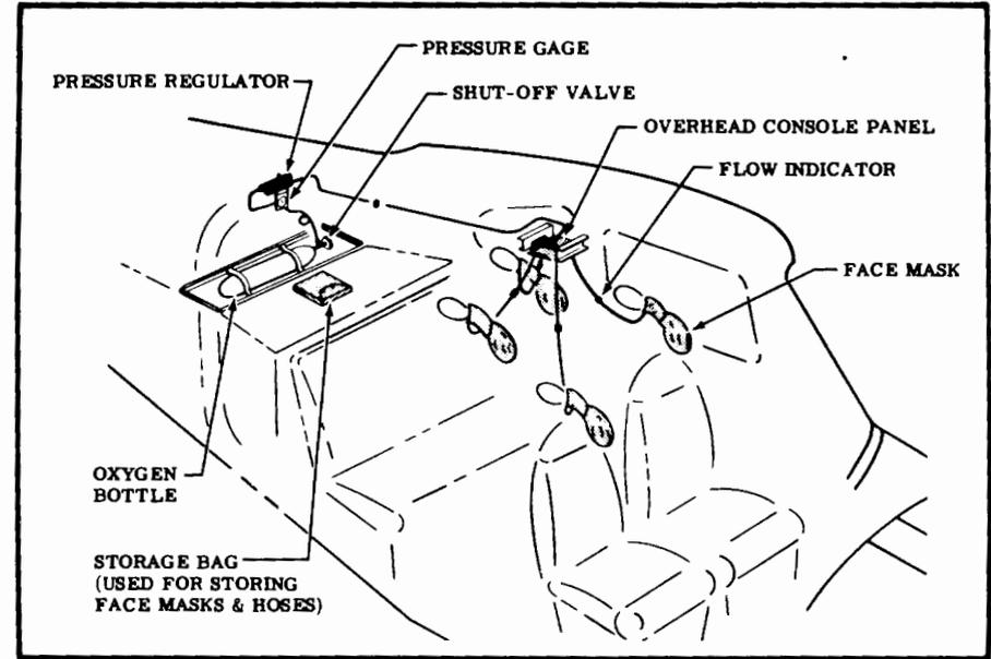
Figure 12. Oxygen System Diagram
