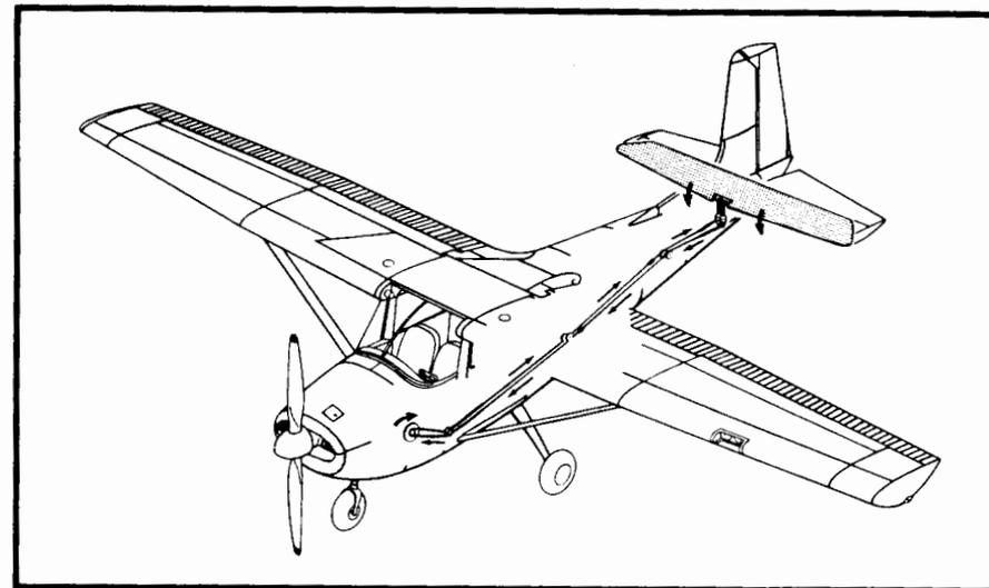
Figure 27. Adjustable Stabilizer Control System
