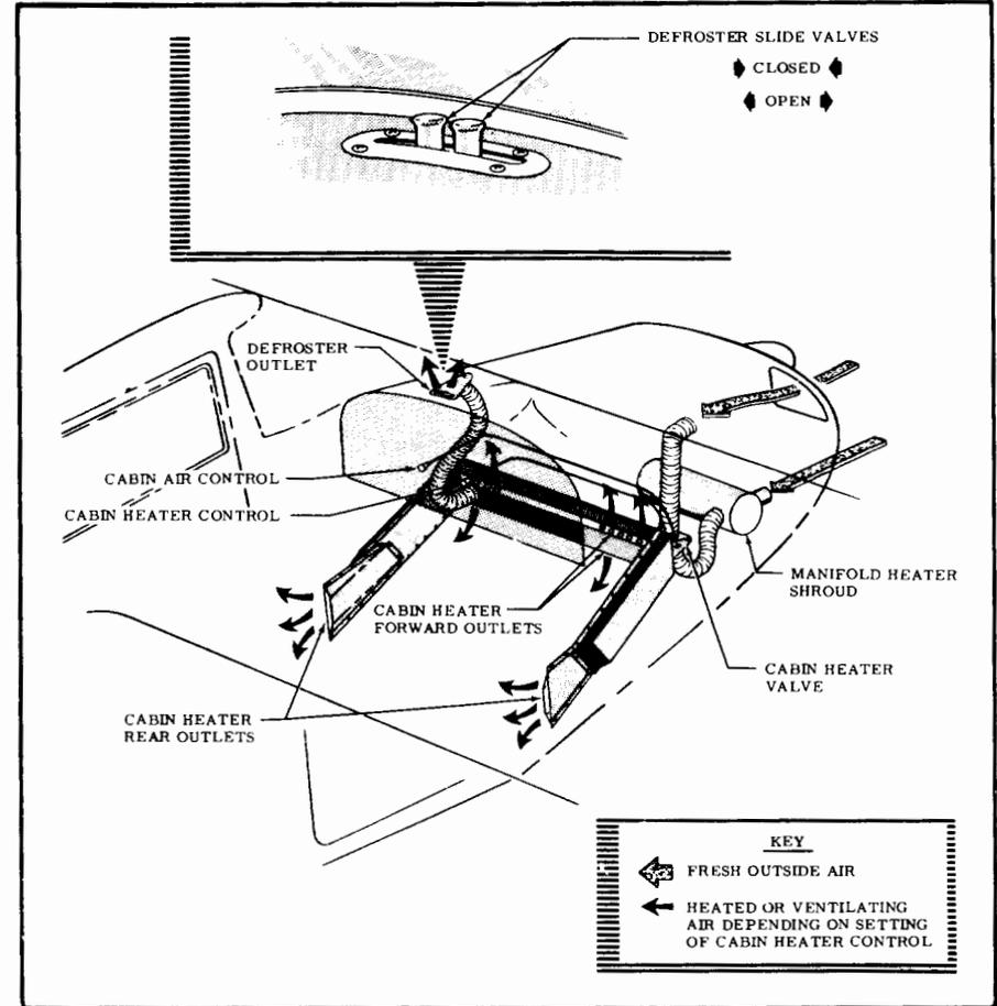
Figure 9. Cabin Air Temperature System
