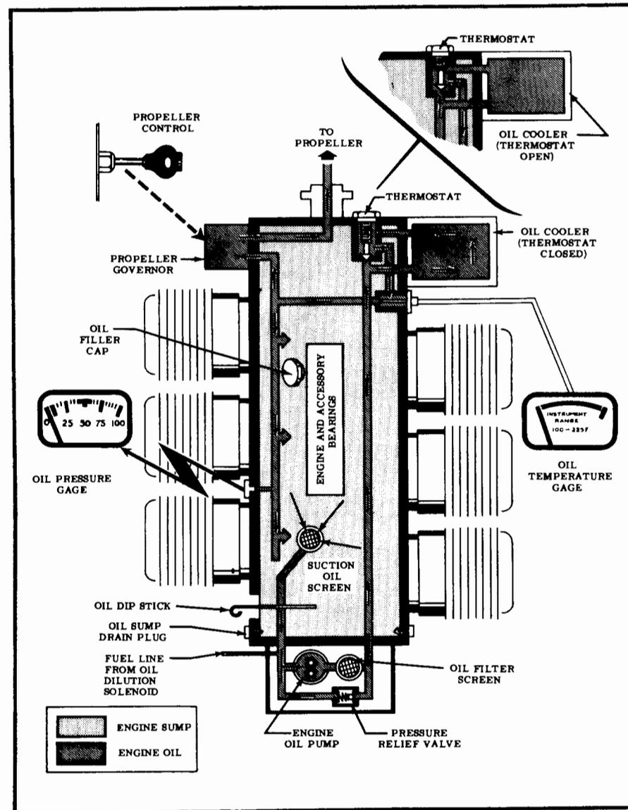
Figure 3. Oil System Schematic
