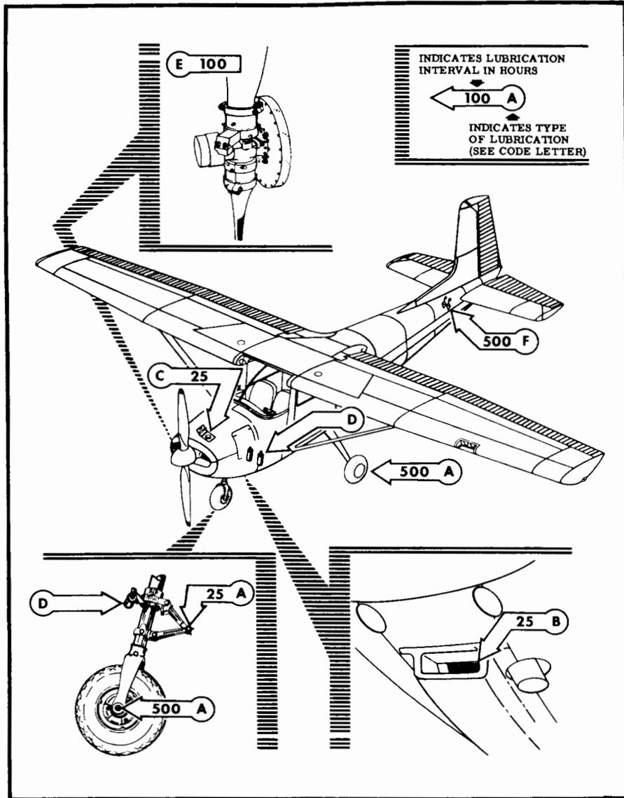
Figure 29. Lubrication Diagram
