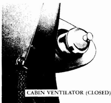
To stop the flow of air, push the ventilator tube all the way in.
